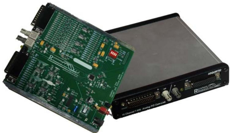
Figure 27. The “ASQUIRT02” 16 channel 1 kHz analog F/O communications link, a sub-unit of the Alcator C-Mod TPS.
