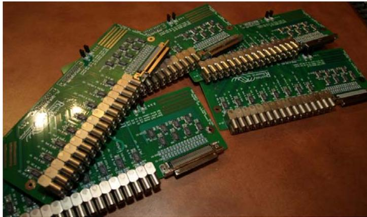
*Figure 5. Five of the analog repeater boards (the third, or top board of the front assembly) are shown above. Analog signals, scaled and buffered are brought onto this board via board-board connectors, repeated via on-board buffers separately to single-pin LEMO test points and to a SCSI168 connector to mate with fast digitizer.*
