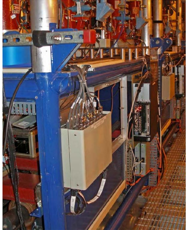
interface was built on two circuit boards which are stacked vertically to give two rows of detectors on opposite faces of a commercial enclosure. The boards are built to “wrap around” the embedded two DSQUIRT digital transceiver boards which link these controls to the PLC.
