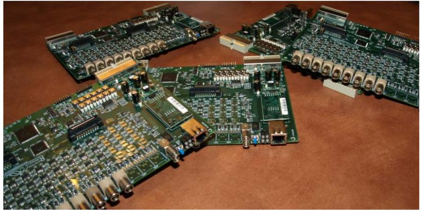
Figure 3. Five of the main boards are shown above. Each of these boards services 12 analog channels (eight body currents, 1 ground current, and 3spares). In addition, there is a repeater port for MDSplus start and clock signals, an Ethernet port, and reset button and LED status display. Both the master CPU and Event Logger CPU, in addition to the programmable fault logic matrix are resident here.
