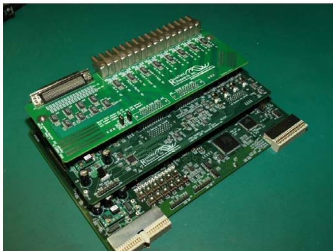
delay after the HV is turned on). The signal is then fed to several analog points of interest: 1) buffered and passed to a dTacq digitizer connector, 2) buffered and passed to a single pin LEMO testpoint, 3) routed to a local 8-channel 12 bit multiplexed digitizer. This last is digitized with a 12 bit scaling of 0-25A. The COTS microprocessor polls each ADC channel at 1 kHz.
