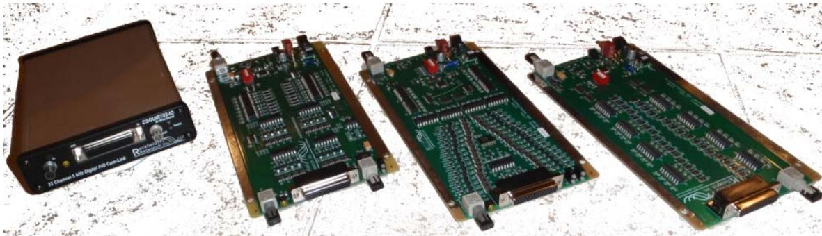
*Figure 28. The DSQUIRT02 digital I/O modules come in three varieties. At left is an “IO” module – 16 channel bidirectional, and next to it is the assembled board for same. Center right is the “OO” module – 32 channel fiber to copper. Far right is the “II” module – 32 channel copper to fiber. Both “II” and “OO” modules assemble into boxes identical to the “IO” assembly shown.*
