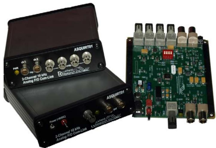
Figure 26. The “ASQUIRT01” 2 channel 10 kHz analog F/O communications link, a sub-unit of the Alcator C-Mod TPS.
