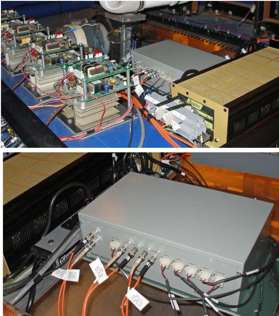
*Figure 19. One of the “box 1 HV control” units is shown installed in the HV area of the cart, adjacent to the legacy filament power supplies, and underneath the klystron sockets.*
