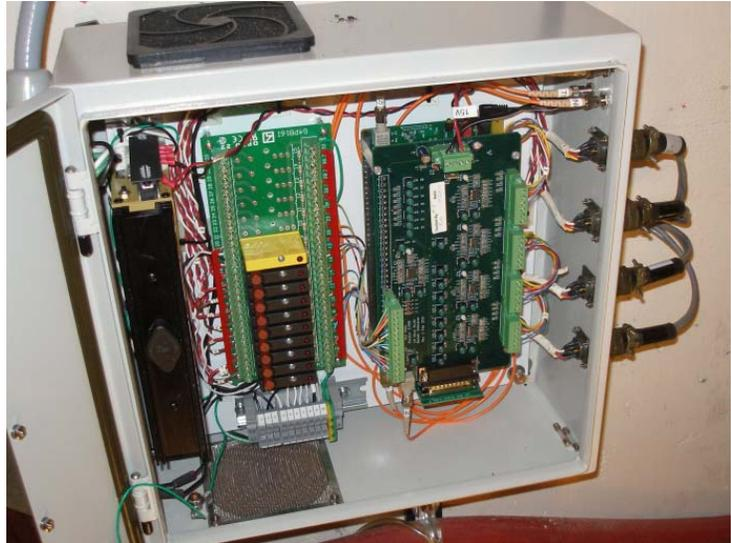
*Figure 20. Each cart has a “box 2 – Waveguide Switch Box”, shown here installed in the C-Mod Cell. Opto-22 interface modules on the left, and a custom interface board at right interface to a DSQUIRT I/O board, mounted underneath at right.*
